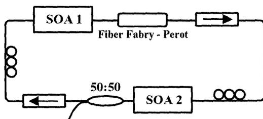
Figure 1: Experimental layout of the multi-wavelength ring laser.
